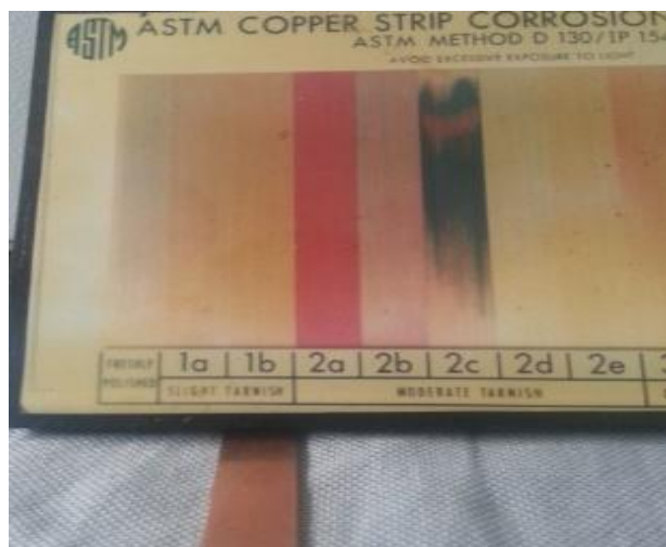
Fig.10. Copper strip corrosion tests of MEO.
