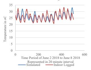
Figure 5: Simulated versus Logged Indoor Temperature graph
