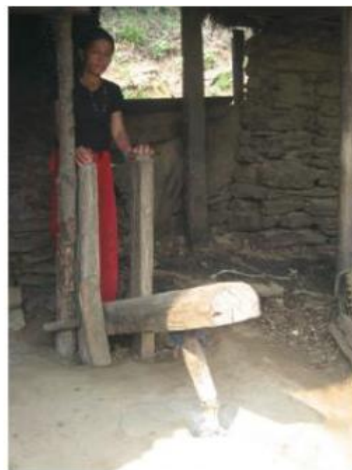
Figure 2. Traditional dehulling equipment, dhiki, being operated by Nepalese woman. (Adapted from Joshi, 2014).
