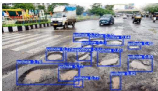
Figure 9: Pothole Detections on Sri Lankan Roads 1
