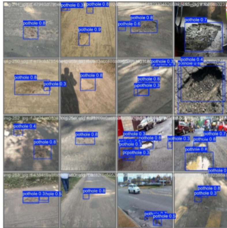
Figure 8: Results of pothole detection
