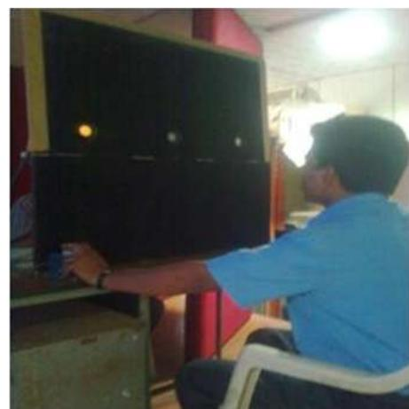
**Fig. 2:** Discrimination Reaction Time (DRT) equipment
