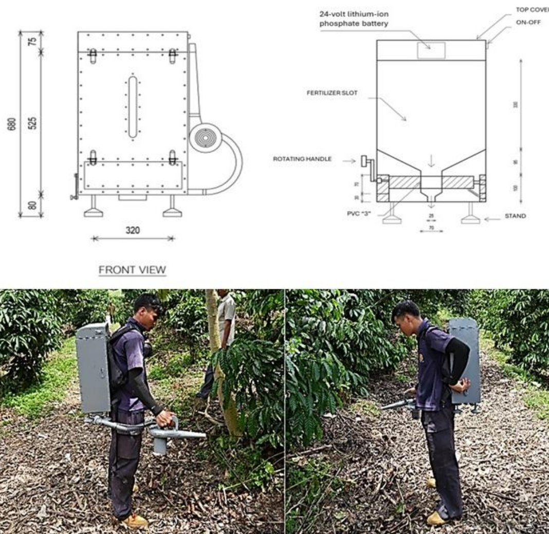
Figure 2: An ergonomic fertilizer applicator prototype simplifies application and reduces farmer strain, proven in field tests
