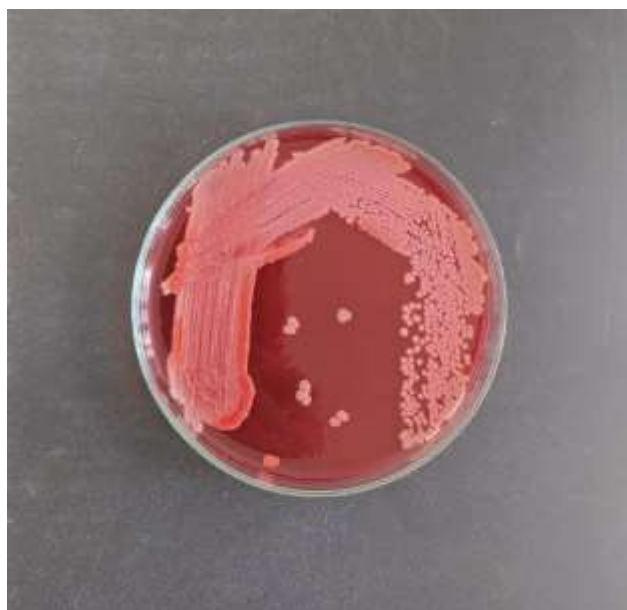
Fig. 2: Congo Red Agar (CRA) plate showing non-biofilm producer with red colonies
