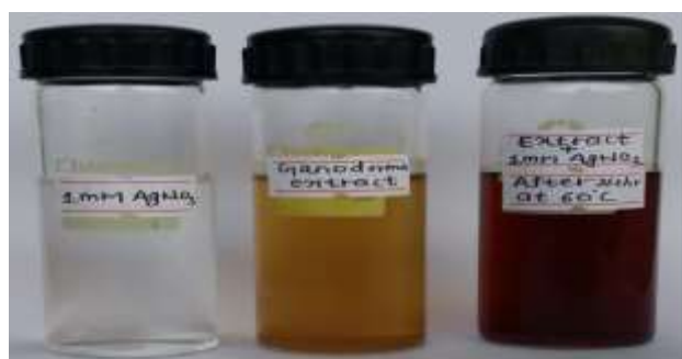
Fig. 1: Color change produced in the silver nitrate solution on addition of Ganoderma extract.
