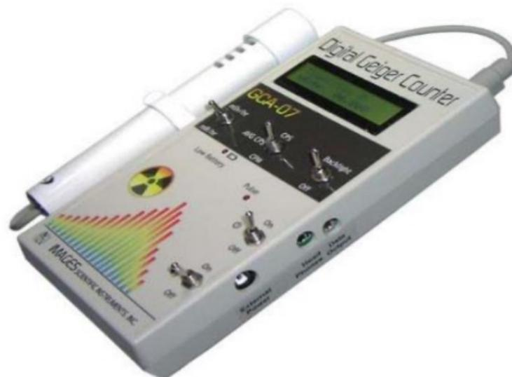
Figure 1. Professional GM counter (GCA-07W) [9], used for measuring the radiation levels.
