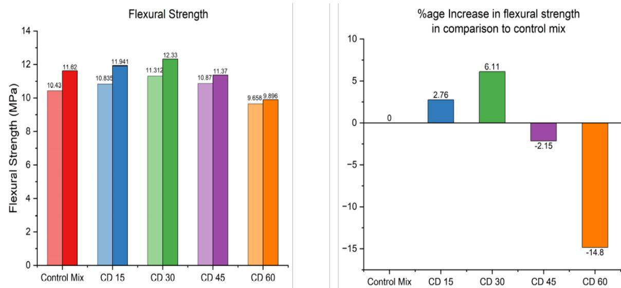
Figure 6: Flexural strength and Percentage increase in flexural strength in comparison to the control mix.
