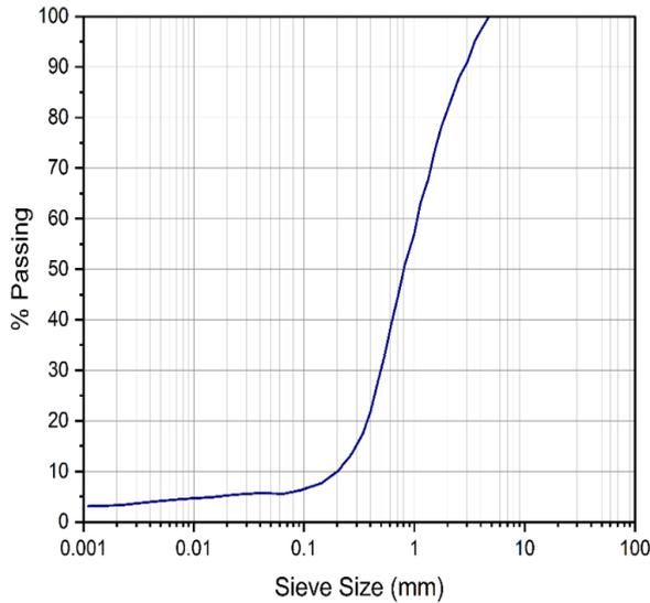
Figure 2: PSD of crusher run dust.
