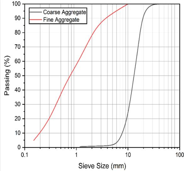
Figure 1: PSD of fine and coarse aggregate.
