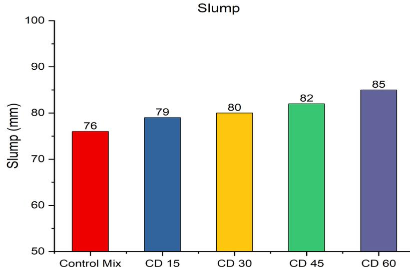
Figure 3: Details of superplasticizer and slump measurement.
