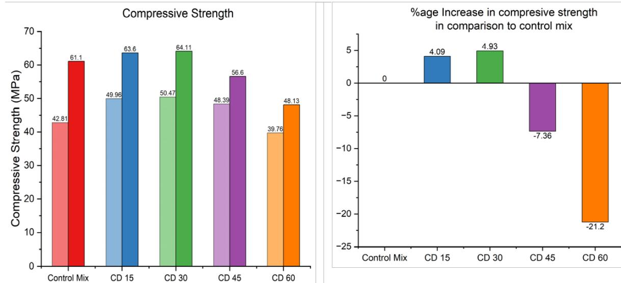
Figure 4: Compressive strength and Percentage increase in compressive strength in comparison to the control mix.
