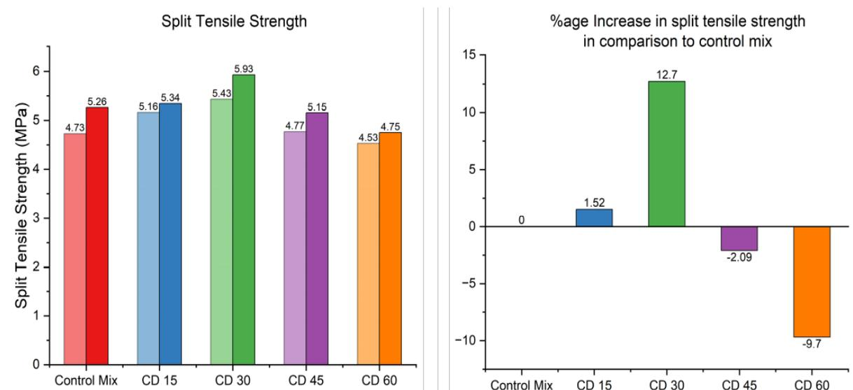
Figure 5: Split tensile strength and Percentage increase in split tensile strength in comparison to the control mix.
