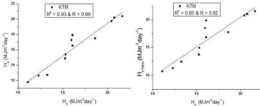
**Figure 3:** Measured ( $\bar{H}_m$ ) versus Estimation global solar Radiation ( $\bar{H}_e$ ) by Angstrom-Prescott model and New model for Kathmandu.
