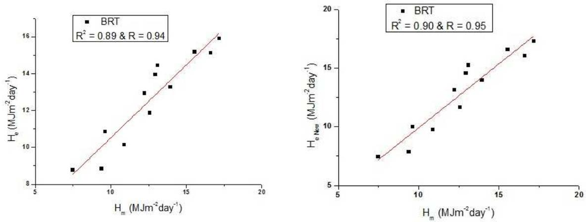
**Figure 2:** Measured ( $\bar{H}_m$ ) versus Estimation global solar Radiation ( $\bar{H}_e$ ) by Angstrom-Prescott model and New model for Biratnagar.
