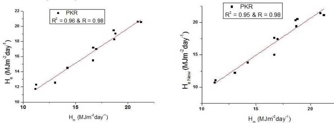
Figure 4: Measured vs Estimation global solar Radiation by Angstrom-Prescott model and New model for Pokhara.
