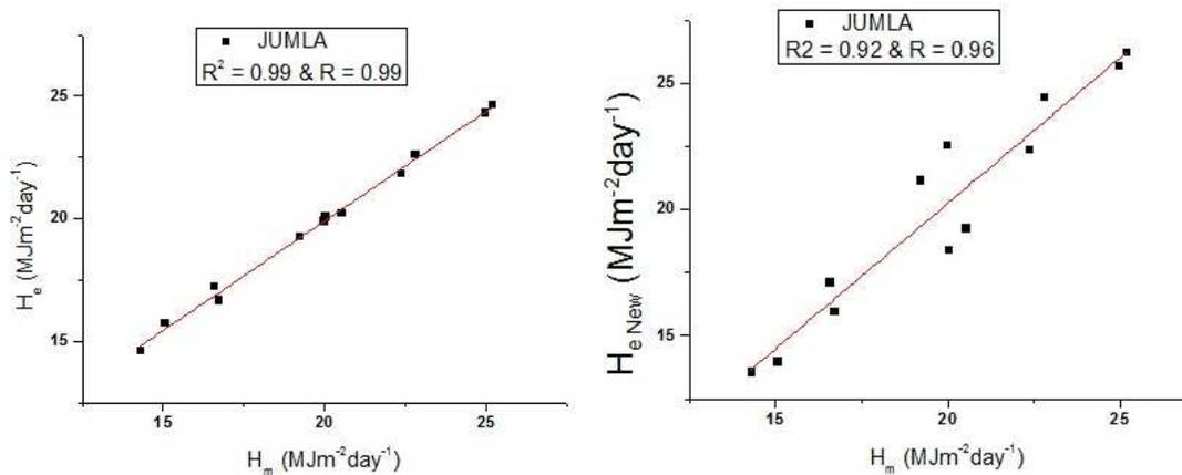
Figure 5: Measured ( $\bar{H}_m$ ) versus Estimation global solar Radiation ( $\bar{H}_e$ ) by Angstrom-Prescott model and New model for Jumla.
